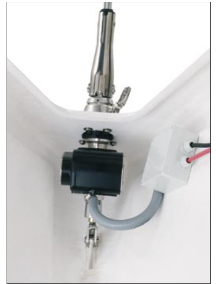
Through-deck installation of a Furler 200E. The connection box is water-tight.
