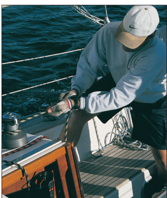
Tension the reef line up to the marked position the line.
