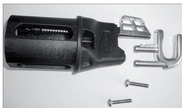
*Remove the two M6 screw inside the pole end.*
