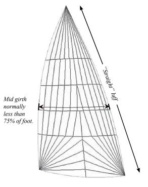
Type of fittings and positions on the mast must be specified by Seldén. In most cases code zero sails need to be hoisted lower than gennakers and spinnakers. Gennaker bow sprits are normally not dimensioned for code zero sails.
