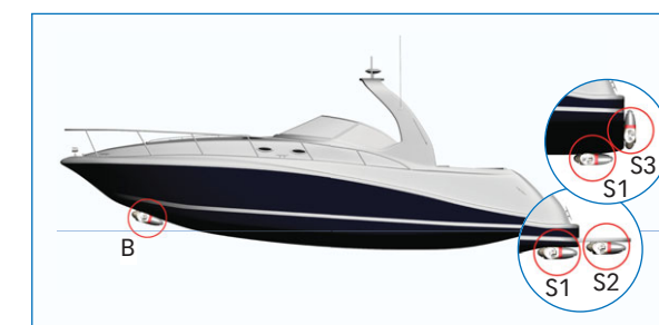
Motorboat B ... mounting as bow thruster Motorboat S1 ... mounting as stern thruster Motorboat S2 ... mounting as stern thruster „bathing platform“ Motorboat S3 ... mounting as stern thruster „vertical transom“
