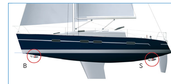
Sailboat B ... mounting as bow thruster Sailboat S ... mounting as stern thruster
