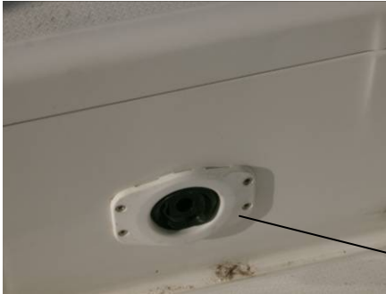
Manual bilge pump, located in the cockpit
