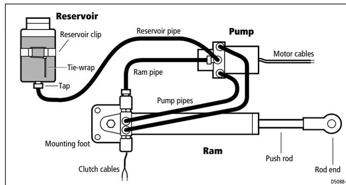
Figure 1: Main components of the hydraulic linear drive system
