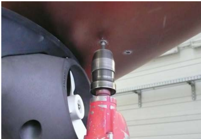
Fig. 24: mounting bolts drilling
