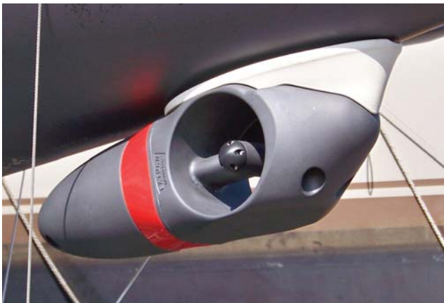
Fig. 27: EXTURN mounted with mounting kit "Adapter"
