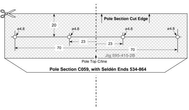
Select correct paper template and cut shaded area. Wrap around one end, align Pole Top Centreline and Section Cut Edge. Mark rivet positions.
