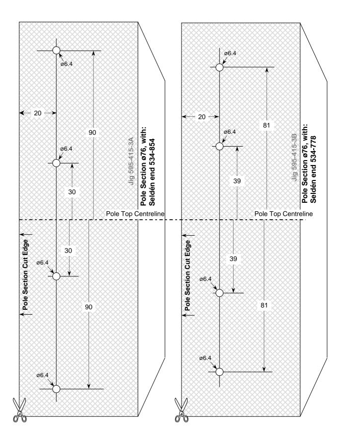
Select correct paper template and cut shaded area. Wrap around one end, align Pole Top Centreline and Section Cut Edge. Mark rivet positions. Repeat at the other pole end
