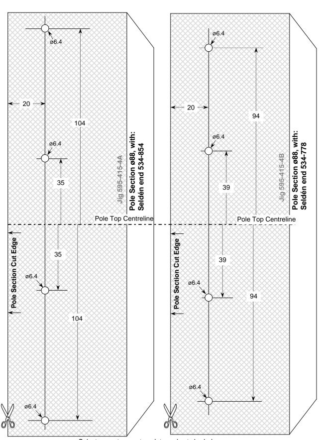
Select correct paper template and cut shaded area. Wrap around one end, align Pole Top Centreline and Section Cut Edge. Mark rivet positions. Repeat at the other pole end
