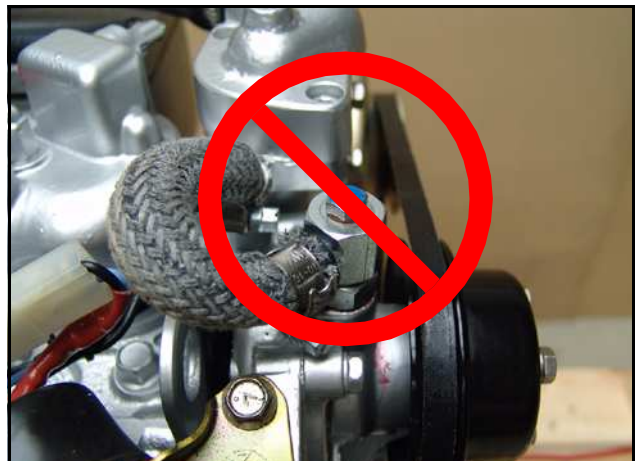
Fig. C.5-5: Vent Screw over the Housing of the Cooling Water Pump
