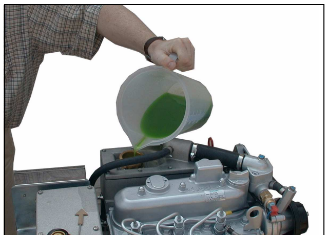
Fig. B.4.2-4: Filling the Cooling Water Circuit
