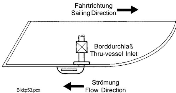
**Never install the thru-hull sea water inlet facing the flow direction.**
