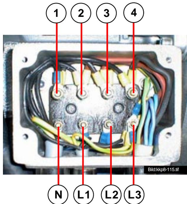
**AC Output terminal box 120V-60Hz.** (shown Panda 8000 with open cover)
