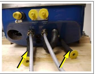
Fig. A.4.3-1: Connection external expansion tank
