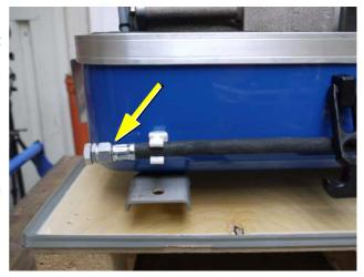
Fig. A.4.8-4: Engine oil drain hose
