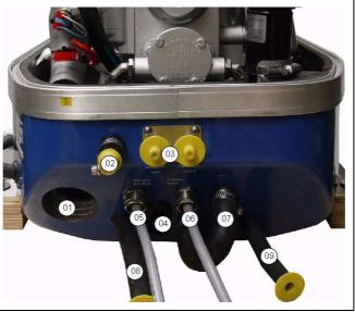
Fig. B.2-2: Connections SCB
