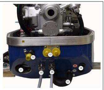
Fig. B.2-1: Connections SCB
