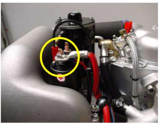
Fig. B.6.1-1: Connection starter battery plus cable
