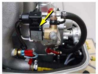
Fig. A.4.5-3: Fuel solenoid valve
