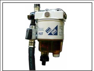
The pre-filter with water separator has a cock at its lower surface, with this cock the downward sunk water can be discharged.
