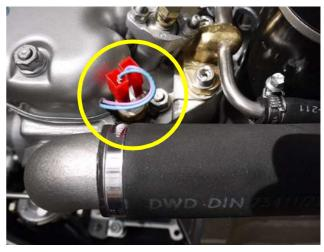
Fig. A.4.7-1: Thermo-switch at cylinder head
