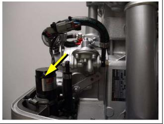
Fig. A.4.3-2: Cooling water pump
