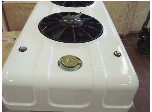
Fig. C.3-4: Cooling water filler cap
