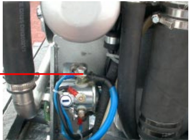
01. Connection positive starter battery cable (+) 02. Connection negative starter battery cable (-)
