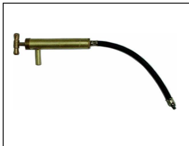
Fig. C.3-3: Oil Drain Pump
