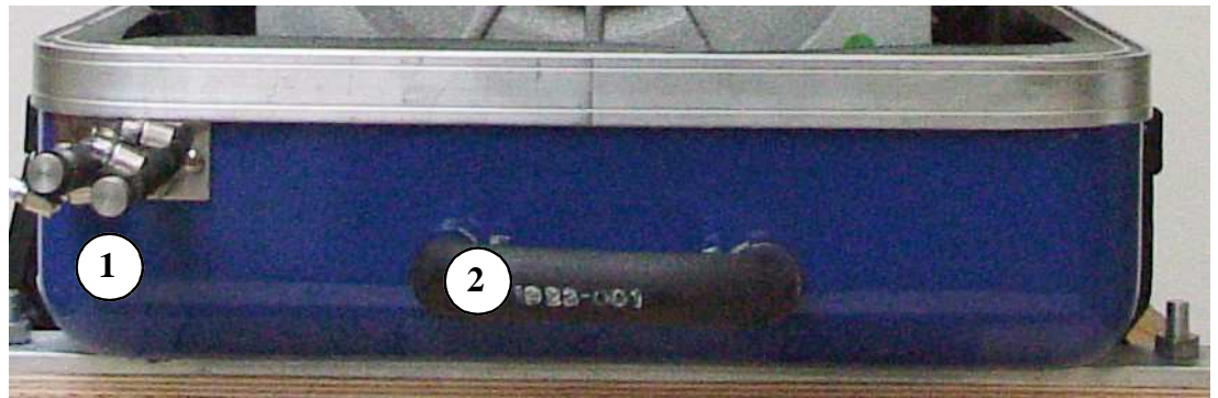
01) external expansion tank
