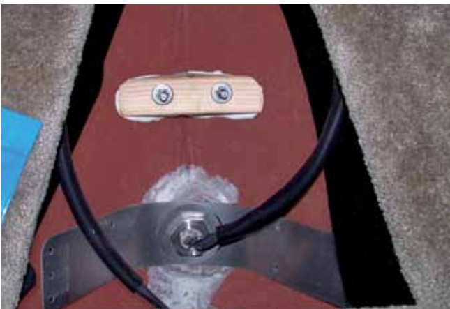
Fig. 25: Screw connection GRP in the boat interior
