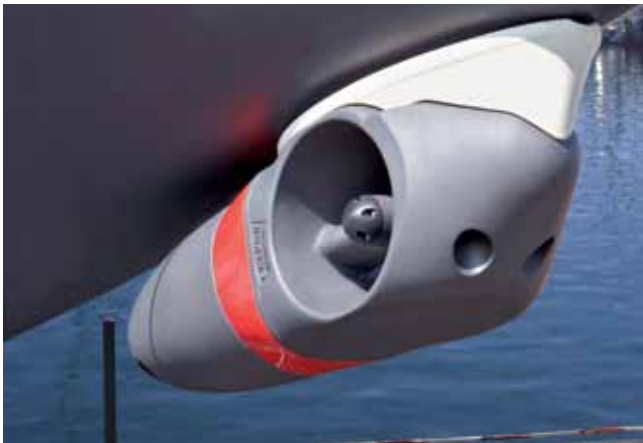
Fig. 22: EXTURN mounted with mounting kit „Adapter“
