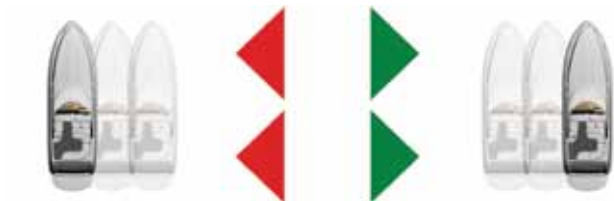
Fig. 44: bow and stern thrusters combined
