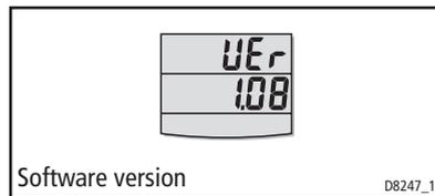
2. Note the software version number, then hold down the **depth** and **speed** buttons for approximately 2 seconds, to return to normal operation.
