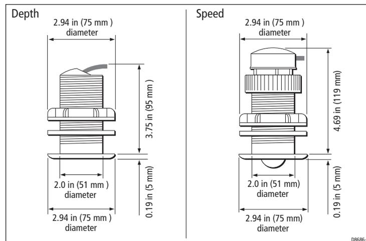
The transducer types required for the various hull types are as follows:
