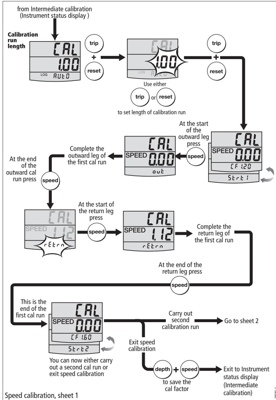
5. At the end of the outward leg, press the **speed** button again so that:
