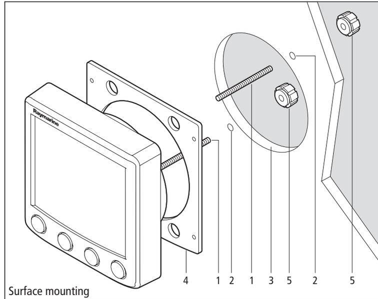
2. Apply the surface mount template (supplied at the rear of this handbook) to the selected location and mark the centres for the fixing studs (1) and the aperture (3) that will take the rear casing of the instrument.
