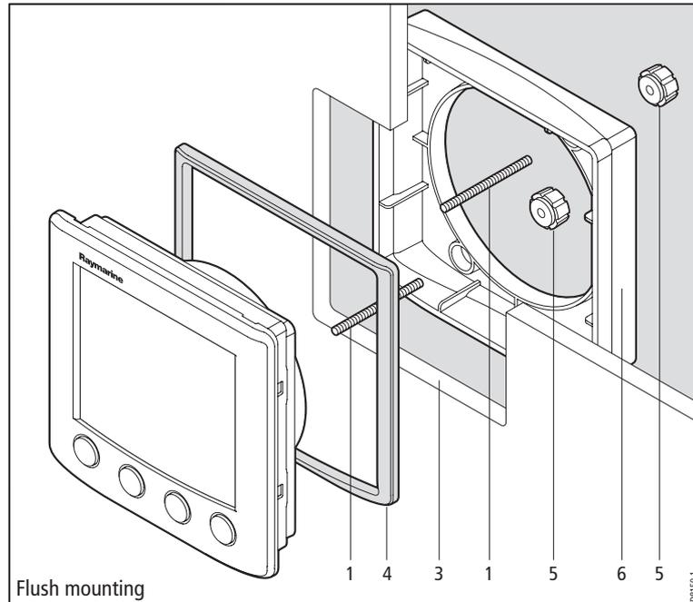
8. Locate the flush mount bracket (6) onto the fixing studs and secure the assembly to the panel with the thumb-nuts (5).
