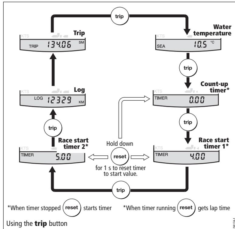
To reset a timer to the start value, stop it then hold down the **reset** button for 1 second.
