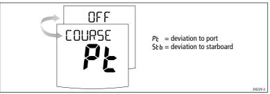
The SmartPilot warns you when you have been off course from the locked heading for longer than 20 seconds. It shows whether the deviation is to port or starboard.
