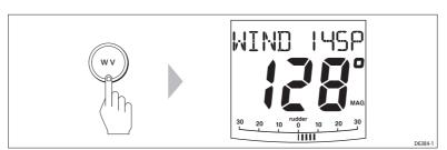
3. In Wind Vane mode, the SmartPilot will then adjust the boat's heading to maintain the locked wind angle.
