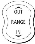
The range of the radar is adjusted by pressing the **RANGE** button.
