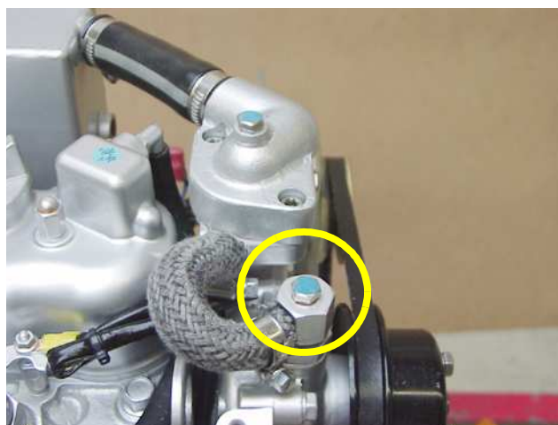
Fig. A.3.2-5: Ventilation screw cooling water pump
