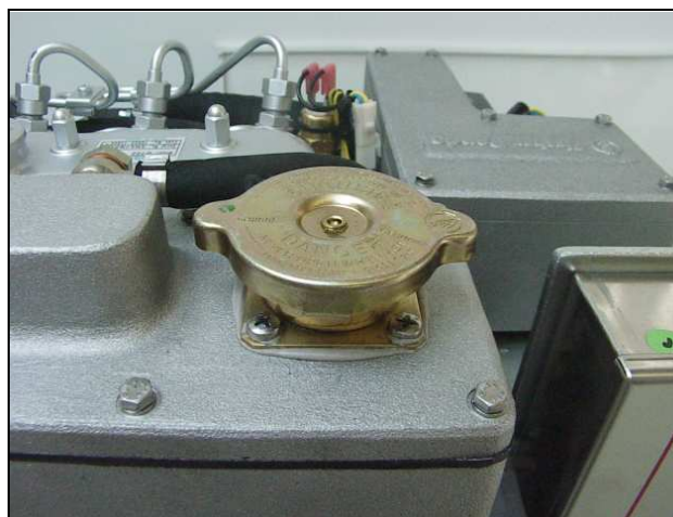
Fig. A.3.2-1: Cooling Water Filler Neck
