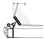
Clew with clew-board: Foot ("E") measured to after point of sail. Clew-board gives longer effective ("E") than integrated block or normal cringle.
