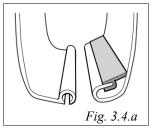
provided (see fig. 3.4.a). If full-length vertical battens are used, round battens generally work better than square battens since square battens can twist. If short vertical battens are used, square battens often work well and are usually less bulky.
