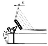
Clew with clew-board: Foot ("E") measured to after point of sail. Clew-board gives longer effective ("E") than integrated block or normal cringle.
