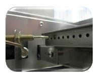
b. Bushman / Bravo – the tip is 2mm from the vertical side of the burner and aligned with the second hole from the end.
