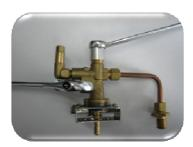
3. Unscrew the aluminum cover. To do this, use a tool to hold the control valve body.
