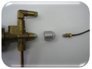
4. The Thermocouple mechanism sits loose in this section. Remove it ensuring that the small rubber seat is on the end of the spring section.
