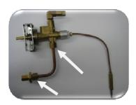
8. Re install the valve into the BBQ. Ensure that the brass inlet fitting is keyed in to the slotted hole in the side of the
