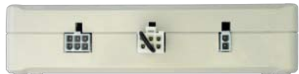
Fig. 39: E-BOX 103 with dummy plug
