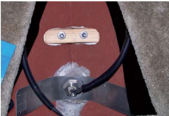
Fig. 31: boat interior bolting GRP
