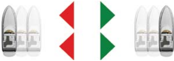
Fig. 44: bow and stern thrusters combined
