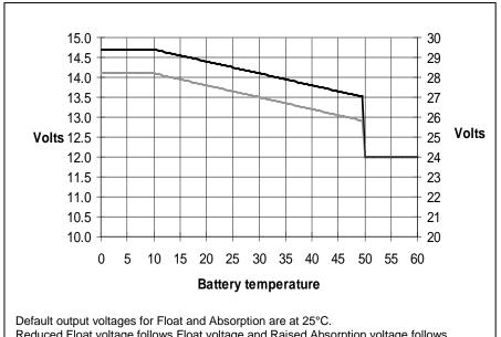
Reduced Float voltage follows Float voltage and Raised Absorption voltage follows Absorption voltage.
