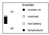
The inverter has switched off due to the electronics temperature being too high.
