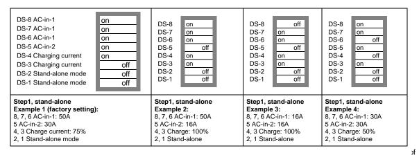
the DIP switches, see appendix A, position K). The overload and low-battery LED's will flash to indicate acceptance of the settings.
