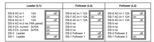
To store the settings after the required values have been set: press the 'Up' button of the **leader** for 2 seconds (**upper** button to the right of the DIP switches, see appendix A, position K). The overload and low-battery LEDs will flash to indicate acceptance of the settings.
