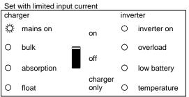
The AC voltage on AC1-in-1 or AC-in-2 is switched through. The AC-input current is equal to the load current. The charger is downcontrolled to 0A.
