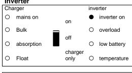
The inverter is on, and supplies power to the load.
