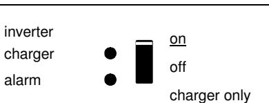
The AC input voltage is switched through and the charger is switched off.
