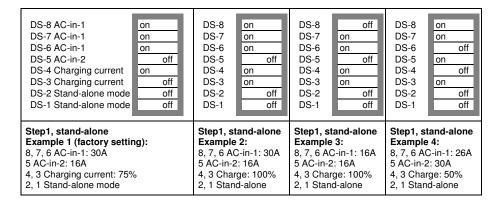
To store the settings after the required values have been set: press the 'Up' button for 2 seconds (**upper** button to the right of the DIP switches, see appendix A, position K). **The overload and low-battery LEDs will flash to indicate acceptance of the settings.**
