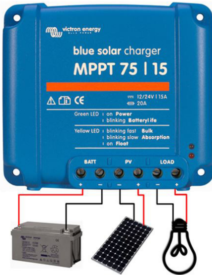
Figure 3: Power connections
