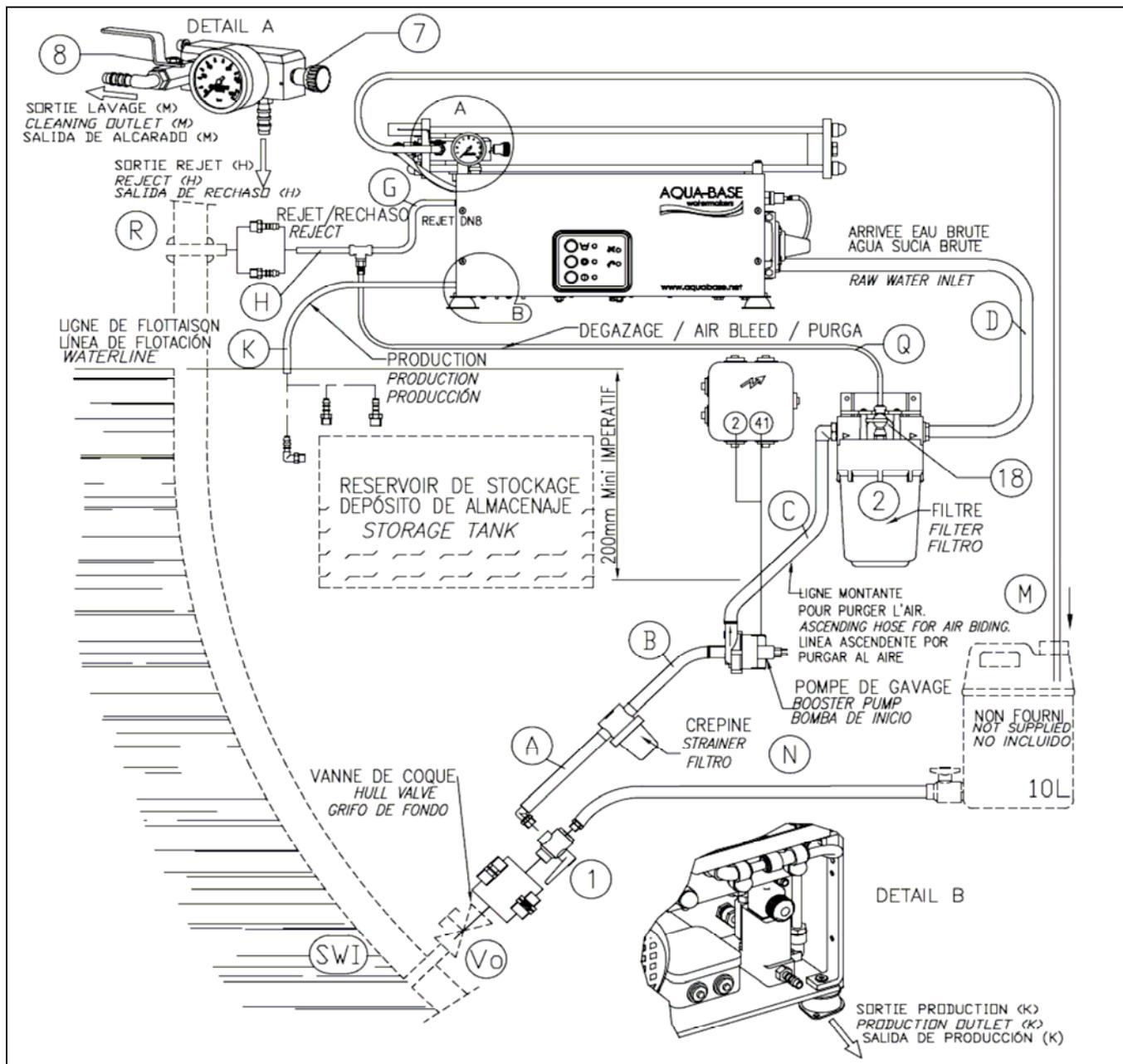
INSTALLATION A BORD AVEC FLUSHING / ON BOARD INSTALLATION LAYOUT WITH FLUSHING /
