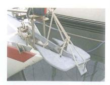
Britain). Brittany anchors are however difficult to stow on the bow roller of most yachts and the model offers no advantage (other than being very cheap) over a Fortress or Danforth. Good in sand and thick mud.
