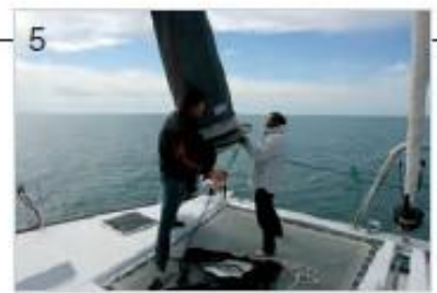
5 Guys and sheets clipped on to their respective points. When you get to know the sail, you can even pre-trim the lines
