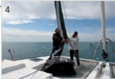
4 Hoist! The spi climbs to the top of the mast, hidden by the sock. A little bit of elbow grease from the crew... or an electric winch!
