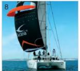
No need for a bowsprit or spi pole here. The deck hardware required is minimal. And gybing is made simple by having a double set of sheets and guys
