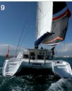
The wing, perfectly trimmed by the multiple hangers, generates a strong lift, great for setting a spi. When unfolded, it also helps the spi maintain a horizontal position
