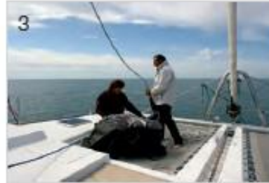
3 The two sheets on each side are ready. The halyard is clipped on to the spi and its sock.
