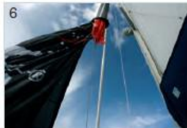
6 With a few tugs, the sock is pulled up to the head of the sail, and the spi fills effortlessly by playing the sheet and guy
