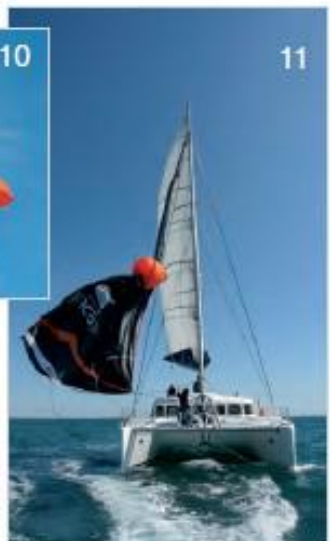
To get it down, all you need to do is pull on the sock's endless line. This operation only slightly slows down as the wing enters the neck of the sock
