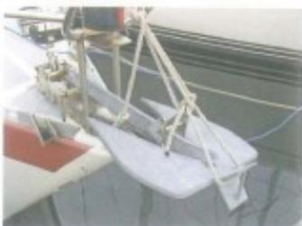
Britain). Brittany anchors are however difficult to stow on the bow roller of most yachts and the model offers no advantage (other than being very cheap) over a Fortress or Danforth. Good in sand and thick mud.
